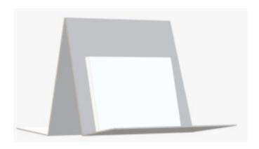
If ALFAPLAS® sheets are stored horizontally, they must not be allowed to sag. Care must be taken to prevent chips or dirt from becoming lodged between the sheets as the weight of the material can force these chips through the protective masking and damage the sheets. If various sizes are stacked horizontally, the larger sheets should be at the bottom to avoid unsupported overhang.
